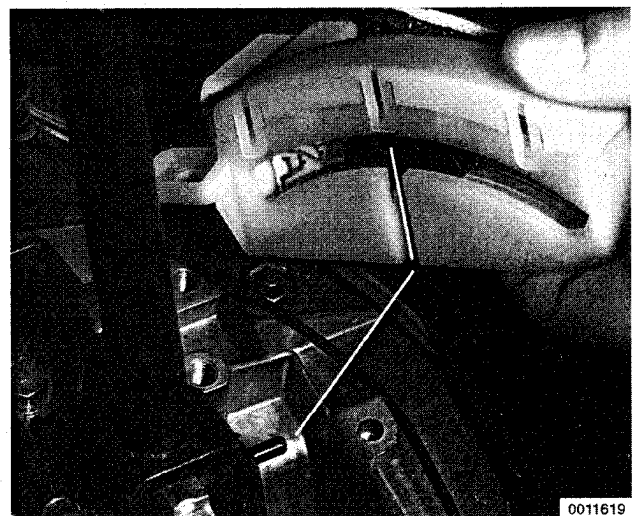
Fig. 9. Contact slide in switch aligns to slot on switch and pin on lever.
