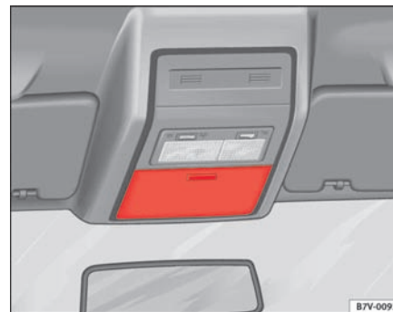
Fig. 104 Stowage area in the roof
