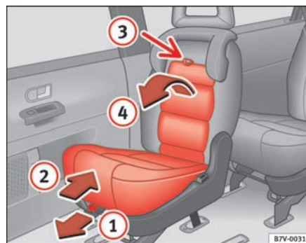
Fig. 35 Using the integrated child seat
