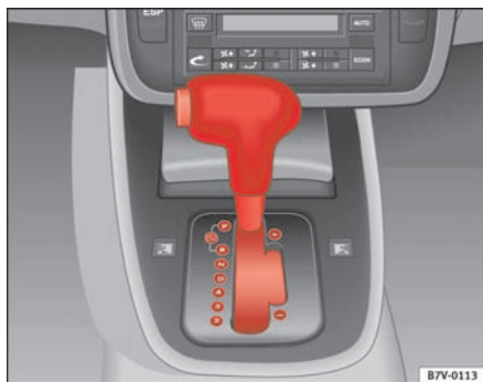
Fig. 130 Section of centre console: selector lever with lock button
