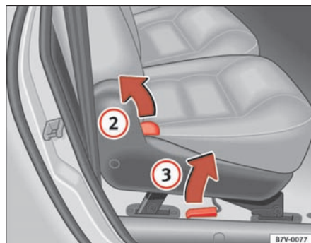
Fig. 91 Side of seat: folding the backrest and raising the seat
