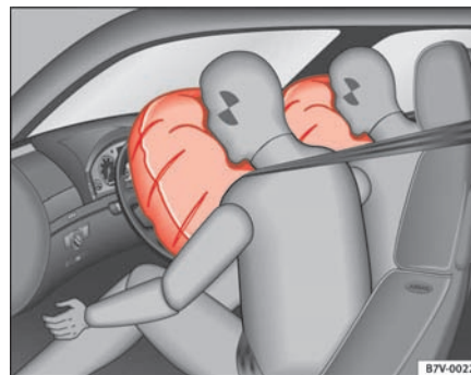
Fig. 24 Inflated front airbags
