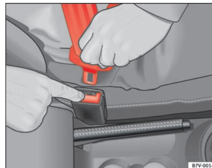
Fig. 16 Removing latch plate from buckle
