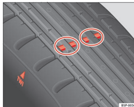
Fig. 150 Tyre tread wear indicators
