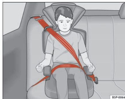
Fig. 32 Forward-facing child seat installed on rear seat.
