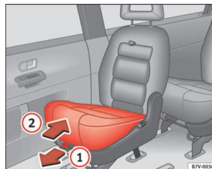
Fig. 40 Fitted child seat: raise the cushion
