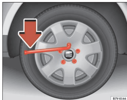
Fig. 159 Changing the wheel: Loosening the wheel bolts
