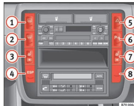
Fig. 79 Centre console: button for thermal windscreen
