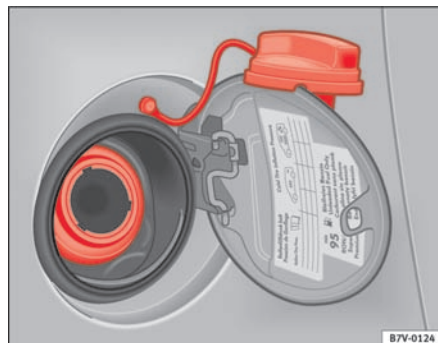
Fig. 138 Tank filler neck and tank flap
