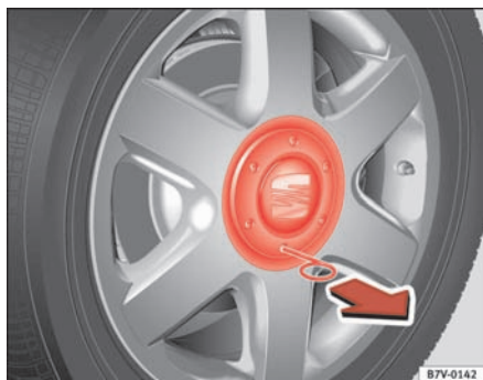
Fig. 157 Removing the hubcaps
