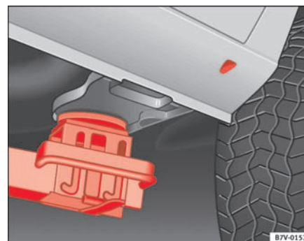
Fig. 177 Lifting with the lifting platform: lifting point at rear left
