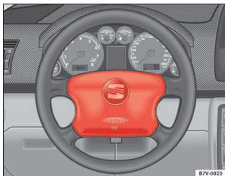
Fig. 22 Driver airbag located in steering wheel
