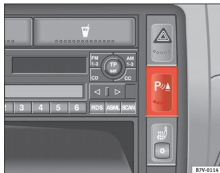
Fig. 132 Section of the dash panel: button for parking distance warning system
