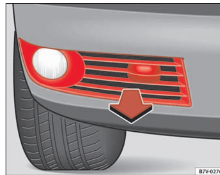
Fig. 174 Towing eye at the front of the vehicle
