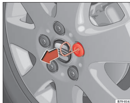
Fig. 158 Use the hook to pull off the cap
