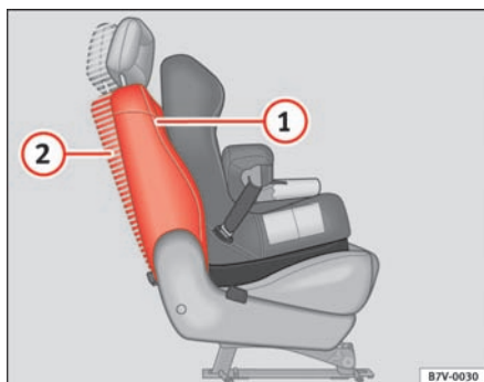
Fig. 34 Backrest adjustment when using ISOFIX child seats
