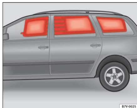
Fig. 27 Deployed curtain airbags
