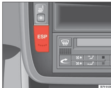
Fig. 125 Section of the dash panel: switch for ESP
