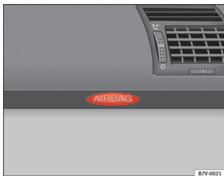
Fig. 23 Front passenger airbag located in dash panel
