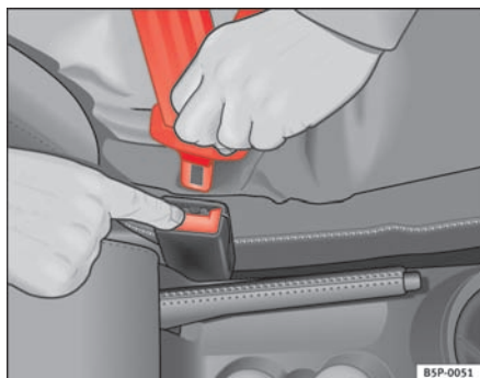
Fig. 15 Removing latch plate from buckle
