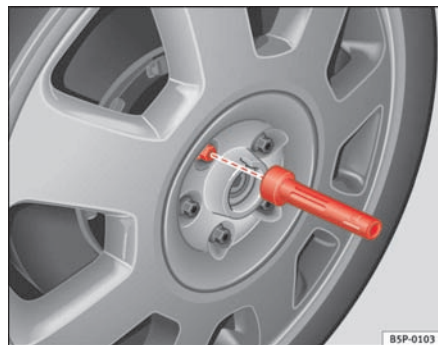
Fig. 125 Changing the wheel: Hexagonal socket in screwdriver handle to turn the wheel bolts
