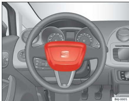
Fig. 16 Driver airbag located in steering wheel
