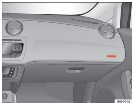
Fig. 17 Front passenger airbag located in dash panel
