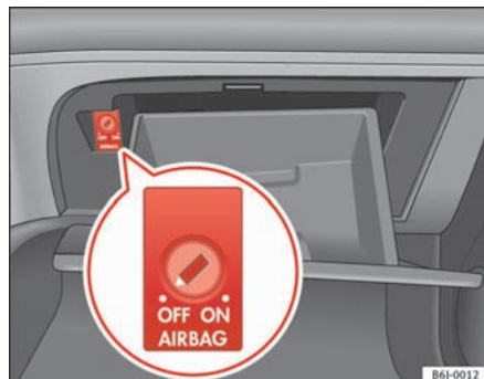
Fig. 23 In the glove compartment: key for enabling and disabling front passenger airbag
