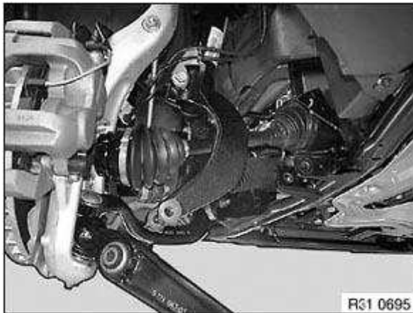
Fig. 120: Moving Steering To Straight-Ahead Position Courtesy of BMW OF NORTH AMERICA, INC.
