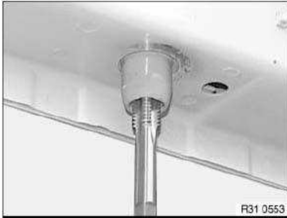
Fig. 9: Creating Thread For Helicoil Thread Insert Courtesy of BMW OF NORTH AMERICA, INC.
