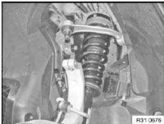
Fig. 56: Identifying Spring Strut Downwards Out Of Wheel Arch Courtesy of BMW OF NORTH AMERICA, INC.
