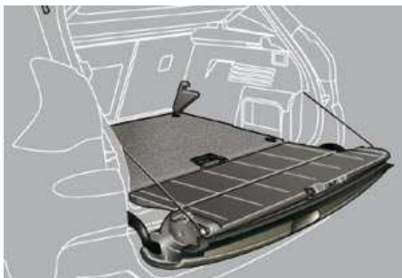
Intermediate position (100 kg max).
