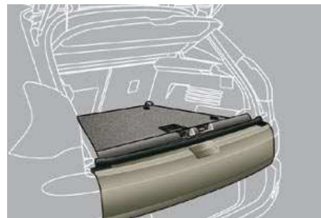
High position (50 kg max) with the lower tailgate closed to isolate the lower part of the boot.
