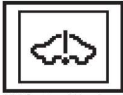
HV System Warning
