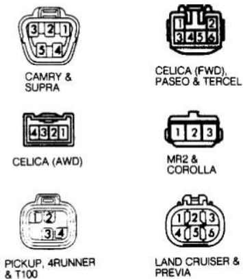
93F84553 Fig. 1: Fuel Sending Unit Harness Connector Terminal ID Courtesy of Toyota Motor Sales, U.S.A., Inc.
