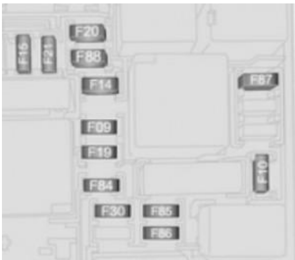
Vauxhall Combo D – fuse box – engine
