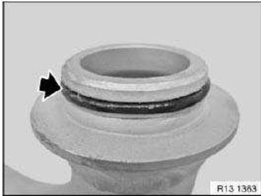
Fig. 76: Locating O-Ring Courtesy of BMW OF NORTH AMERICA, INC.
