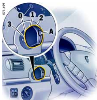
Ignition lock positions with Porsche Entry & Drive: 0 - Initial position 1 - Ignition on 2 - Start engine 3 - Ignition off
