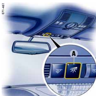
A - Button for dimming the comfort lighting
