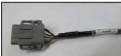
Scrutineering Logger Connector: DTM06-BS
