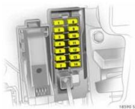
Vauxhall Corsa D – fuse box – passenger
