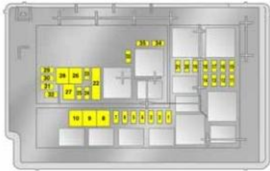
Vauxhall Corsa D – fuse box – engine compartment
