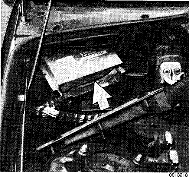
Fig. 42. Engine control module (ECM) located in compartment in right-rear of engine compartment (arrow).
