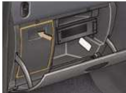
Fascia fuse box
