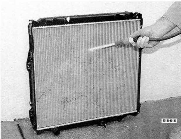
Cleaning the radiator core externally.
