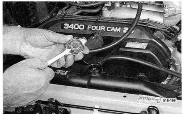
Check the radiator cap sealing rubber for deterioration.
