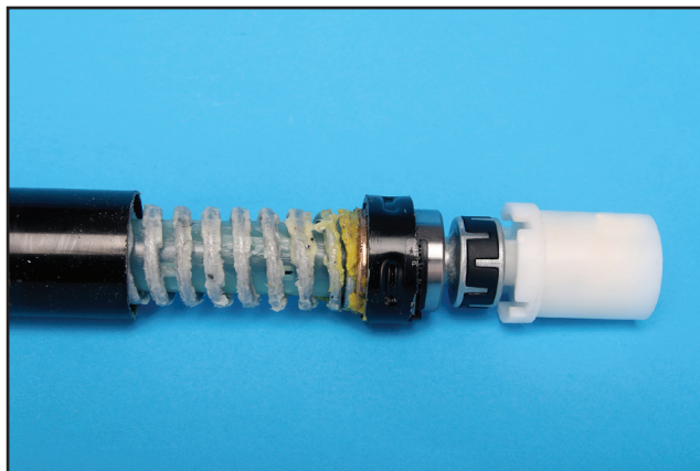
Figure 5-77 PRG gate stay assist spring, motor drive damper, and planetary gearset
