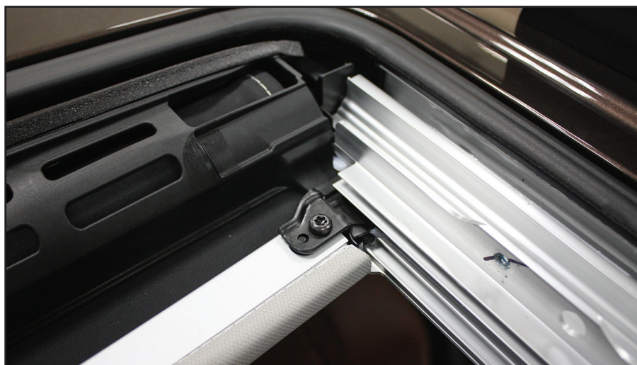
Figure 6-4 Screw Connecting the Shade to Moonroof Track
