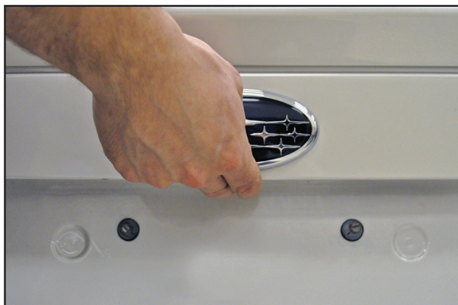
Figure 1-81 Driver Touching Trunk Switch
