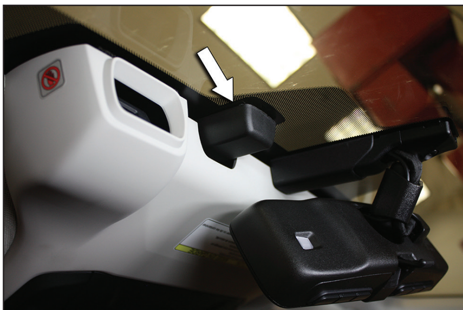
Figure 8-2 Rain Sensor (Center)
