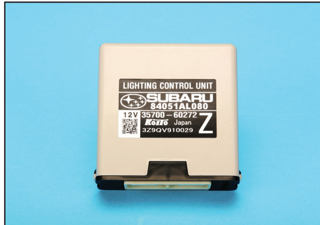
Figure 3-42 Lighting Control Unit
