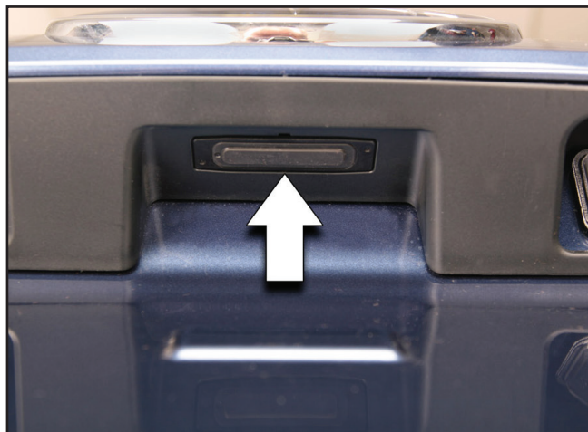
Figure 5-3 Gate Opener Switch
