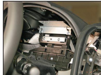
Figure 2-81 Sub Antenna Location
