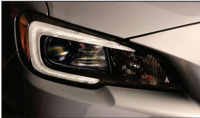
Figure 3-19 LED Parking Lamp
