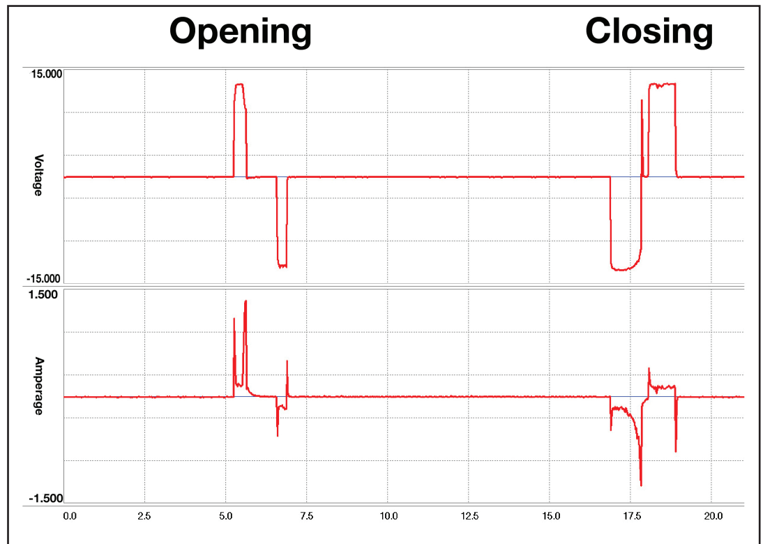
Figure 5-86 PRG Auto Closer Voltage and Amperage
