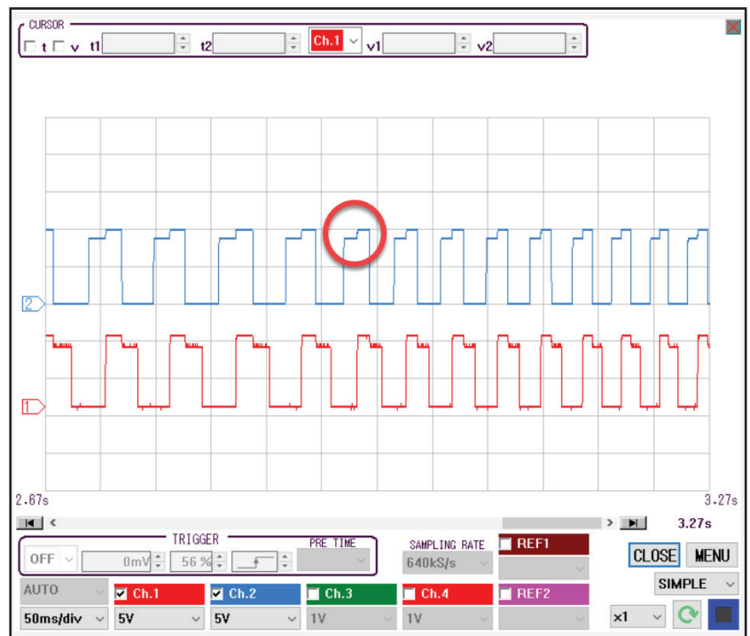
Figure 5-80 PRG position sensor Hall 1 and 2 – Closing
