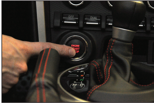
1. The driver sits in the driver seat. The interior antenna transmits a signal to the remote key. The remote key transmits a signal to the receiver. 2. The driver presses the Engine Start and Stop button once with their foot off of the brake pedal. The accessory position circuit turns on and allows operation of all accessory circuit devices.
