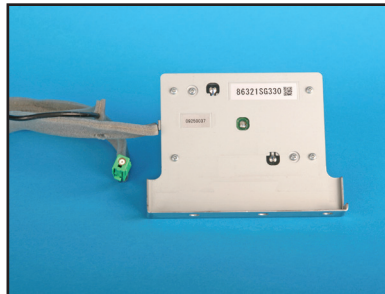
Figure 2-80 Sub Antenna-Removed (Bottom)
