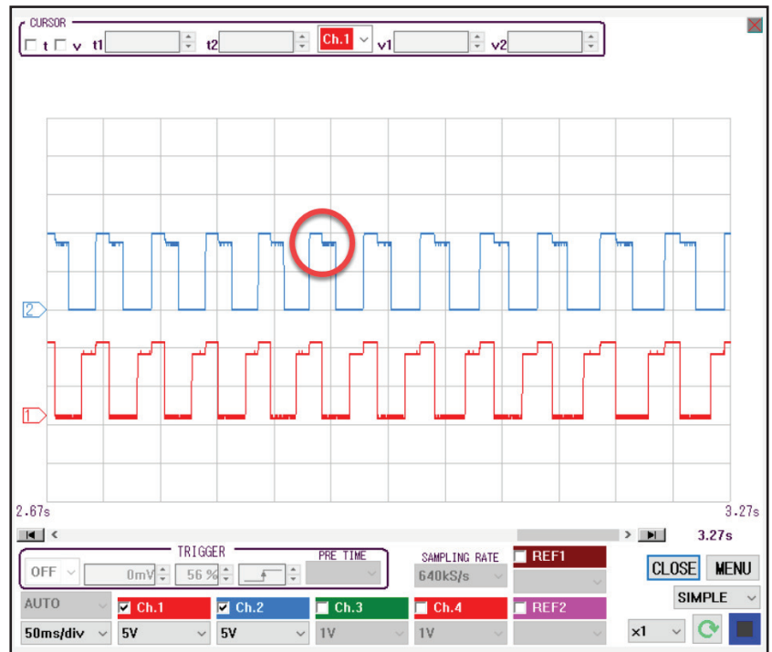
Figure 5-79 PRG position sensor Hall 1 and 2 – Opening
