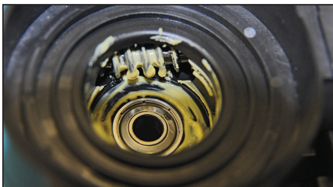
Figure 5-24 PRG Drive Unit Motor Coupling Gear
