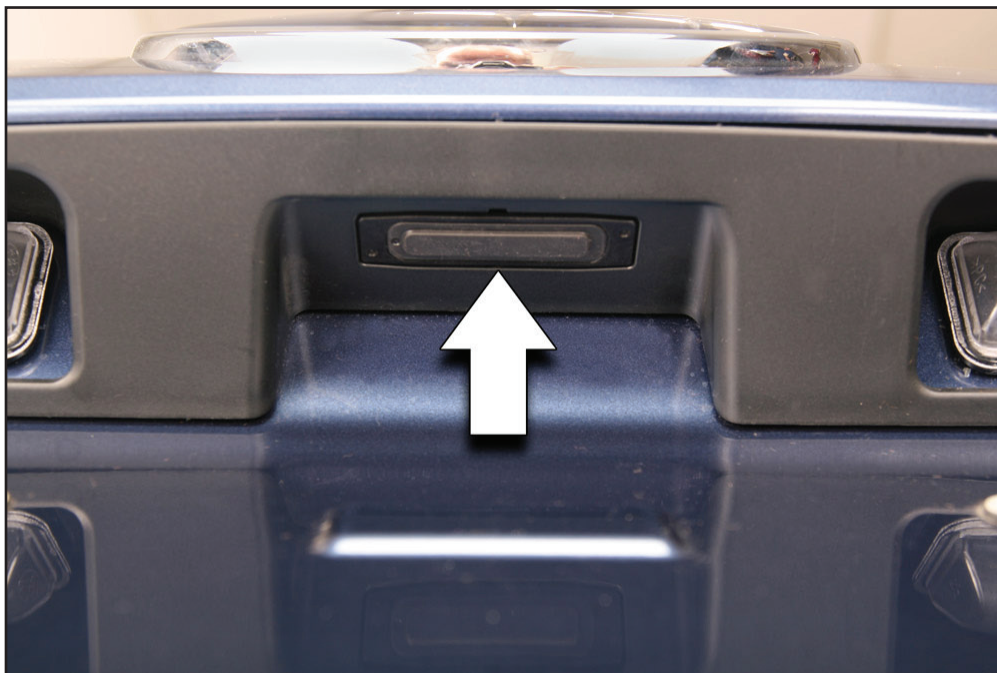
Figure 5-38 Gate Opener Switch
