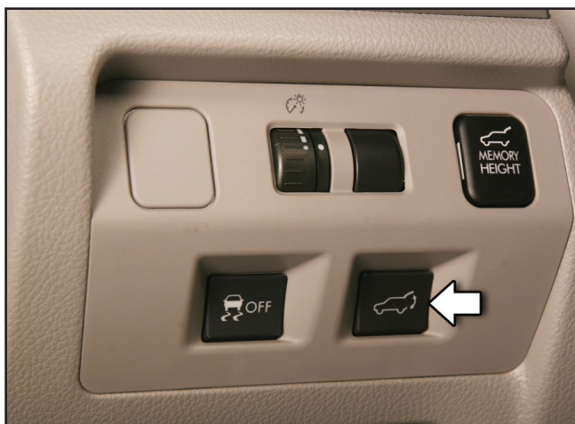
Figure 5-6 Interior PRG Open/Closer Switch
