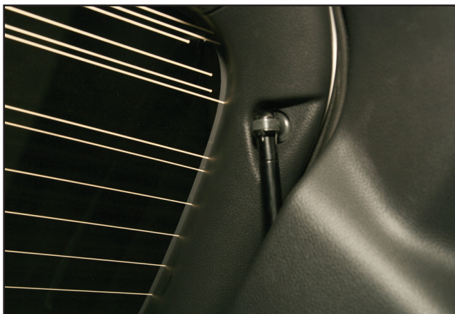
Figure 5-69 Top of Gate Lift Arm Gate Closed
