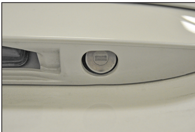
Figure 1-84 Trunk Mechanical Key Slot
