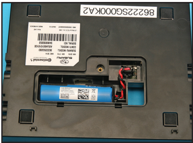
Figure 2-72 Back-up Battery (BUB)
