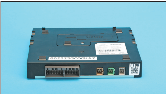
Figure 2-67 Data Communication Module (DCM)
