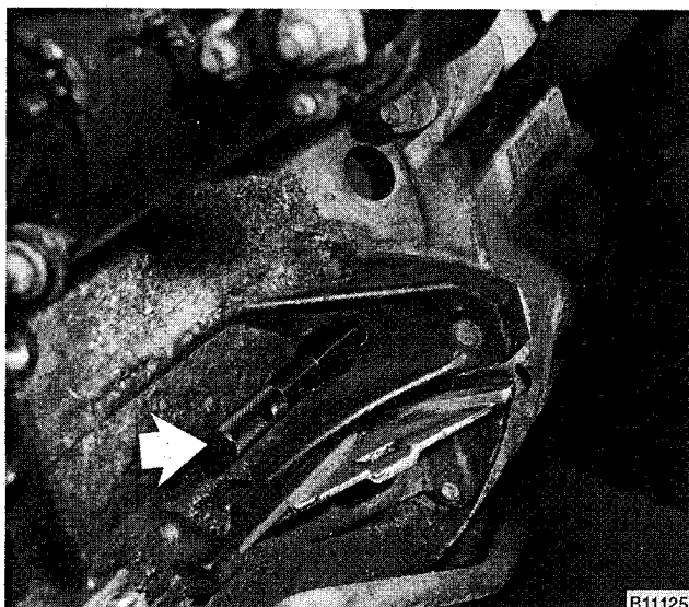
Fig. 11. BMW special tool no. 11 2 300 installed through bellhousing and into flywheel (arrow) to lock crankshaft at TDC.
