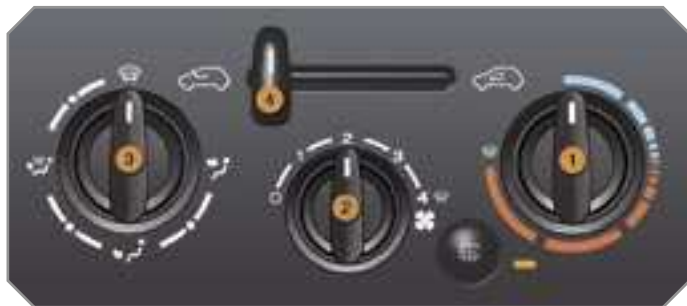
Control panel with manual control
