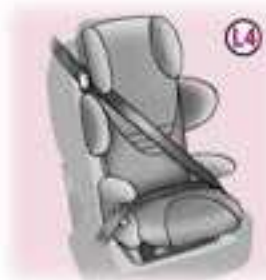
L4 - "RECARO Start": installed using a three-point seat belt.
