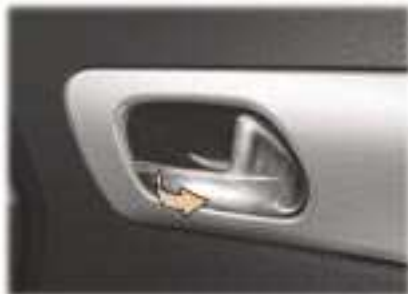
Opening the doors from inside
