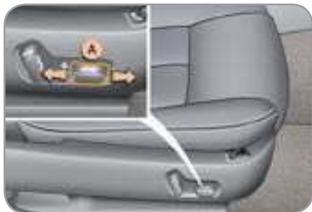
A. Forwards-backwards adjustment.
