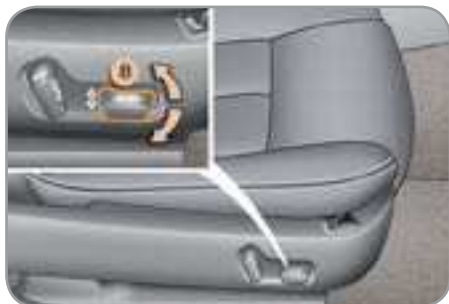
B. Seat cushion angle adjustment.
