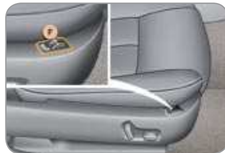
F. Heated seats adjustment.
