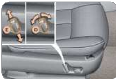
D. Seat back angle adjustment.
