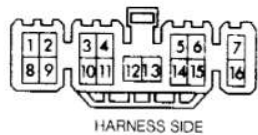
Fig. 3: Power Door Lock Harness & Connector Circuit Testing Courtesy of Toyota Motor Sales, U.S.A., Inc.
