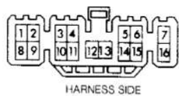
93H84407 Fig. 2: Power Door Lock Harness & Connector Circuit Testing Courtesy of Toyota Motor Sales, U.S.A., Inc.
