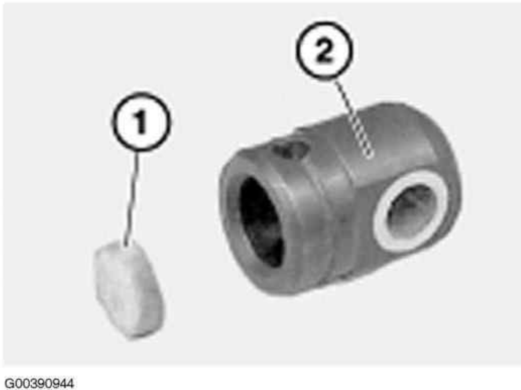
Fig. 39: Checking Rubber Ring In Shift Rod Joint Courtesy of BMW OF NORTH AMERICA, INC.
