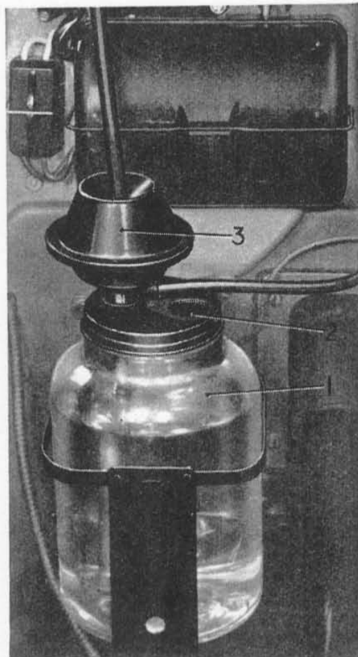
Fig. 49.—RESERVOIR AND PUMP.
