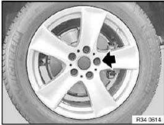
Fig. 126: Locating Wheel Bolt
