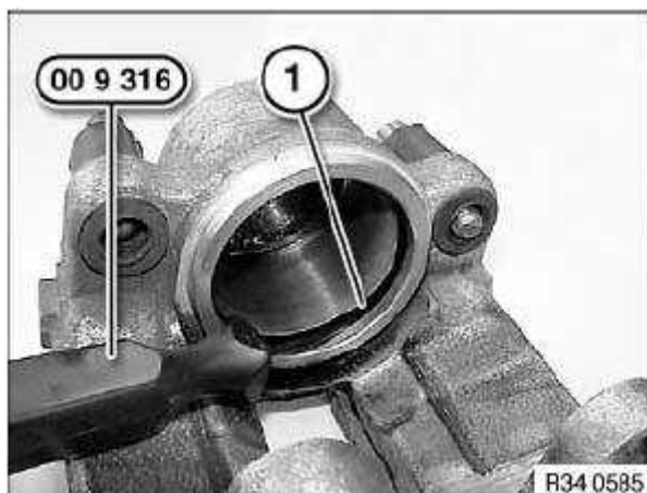
Fig. 89: Removing Seal With Special Tool (00 9 316)
