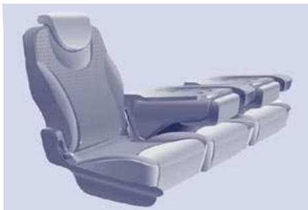
Type 2: two seats with folding seat backs and seat cushion which can be raised.
