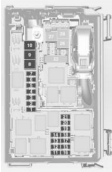
Vauxhall Meriva B – fuse box – engine compartment
