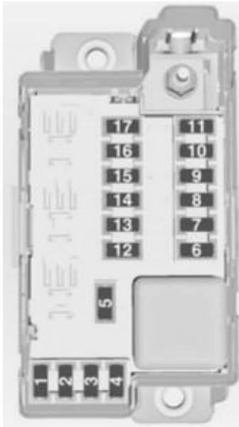
Vauxhall Meriva B – fuse box – load compartment
