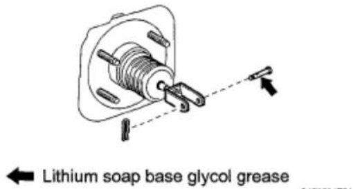
Fig. 36: Applying Lithium Soap Base Glycol Grease To Push Rod Pin Courtesy of TOYOTA MOTOR SALES, U.S.A., INC.
