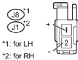
Front view of wire harness connector: (to Rear No. 3 Speaker)
