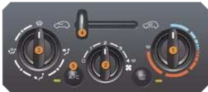
Control panel with manual control
