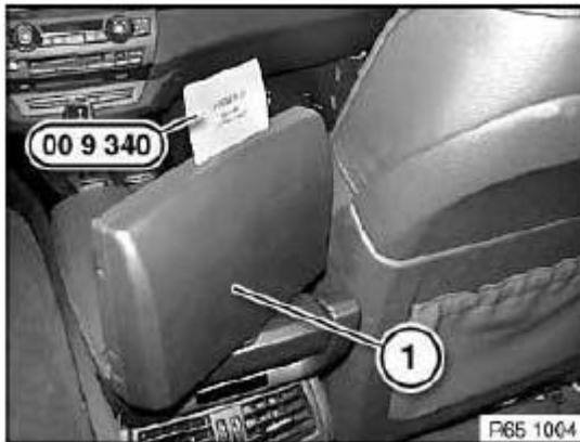
Fig. 47: Identifying Special Tool (00 9 340) On Trim Courtesy of BMW OF NORTH AMERICA, INC.
