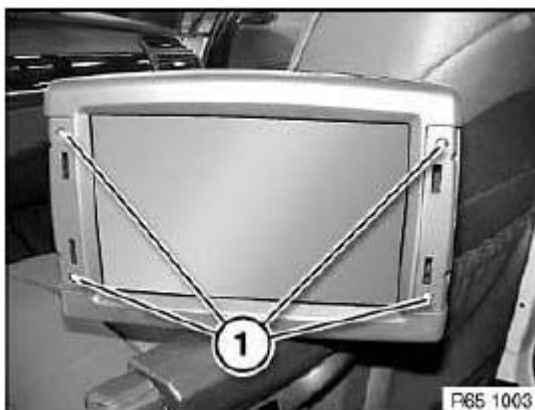
Fig. 46: Identifying Trims Screws Courtesy of BMW OF NORTH AMERICA, INC.
