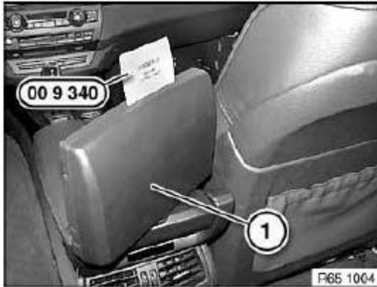
Fig. 51: Identifying Special Tool (00 9 340) On Trim Courtesy of BMW OF NORTH AMERICA, INC.
