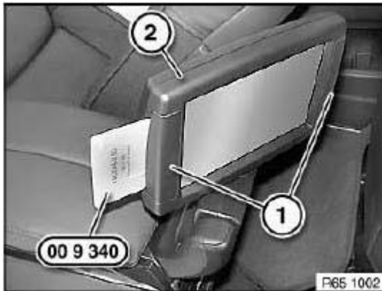
Fig. 49: Identifying Special Tool (00 9 340) On Trims Courtesy of BMW OF NORTH AMERICA, INC.
