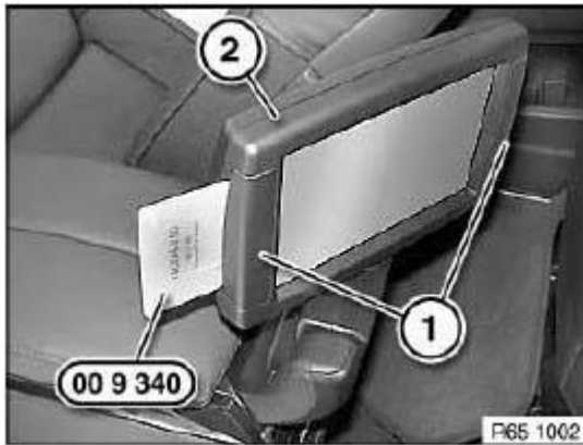
Fig. 45: Identifying Special Tool (00 9 340) On Trims Courtesy of BMW OF NORTH AMERICA, INC.
