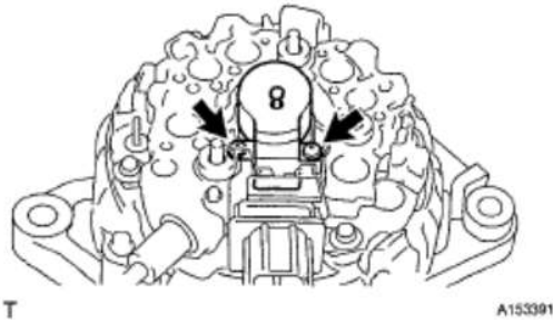
Fig. 47: Locating Generator Coil With Screws Courtesy of TOYOTA MOTOR SALES, U.S.A., INC.
