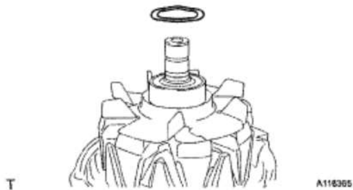
Fig. 43: Identifying Generator Washer On Generator Rotor Courtesy of TOYOTA MOTOR SALES, U.S.A., INC.
