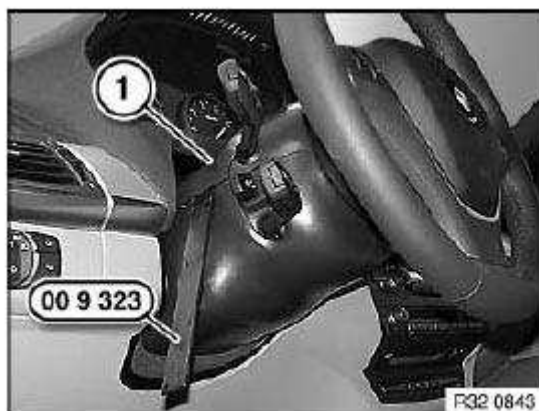
Fig. 43: Uncoupling Steering Column Trim With Special Tool (00 9 323)
