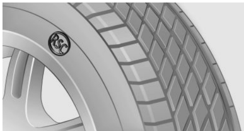
RSC label on the tire sidewall.
