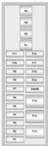
Vauxhall Ampera – fuse box – instrument panel (right side)
