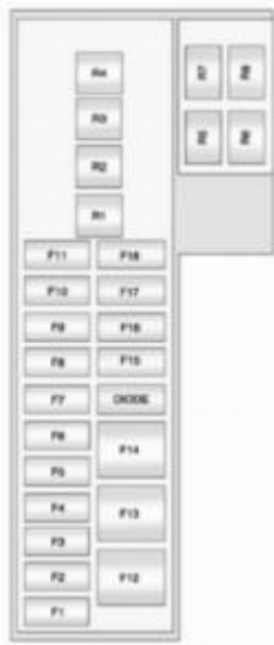
Vauxhall Ampera – fuse box -load compartment
