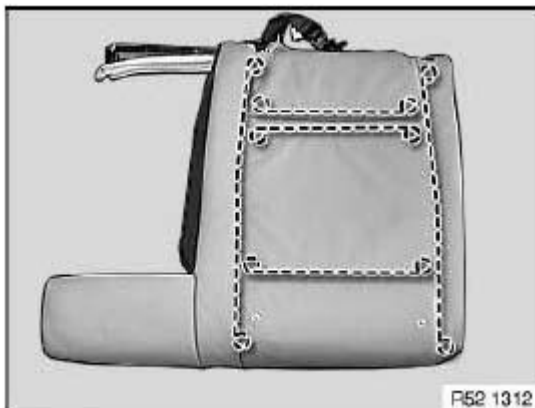
Fig. 174: Identifying Trim Wires Into Cover Pockets Courtesy of BMW OF NORTH AMERICA, INC.
