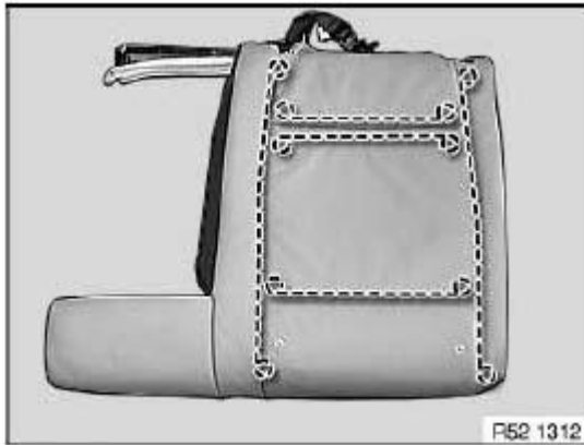
Fig. 180: Identifying Trim Wires Into Cover Pockets Courtesy of BMW OF NORTH AMERICA, INC.
