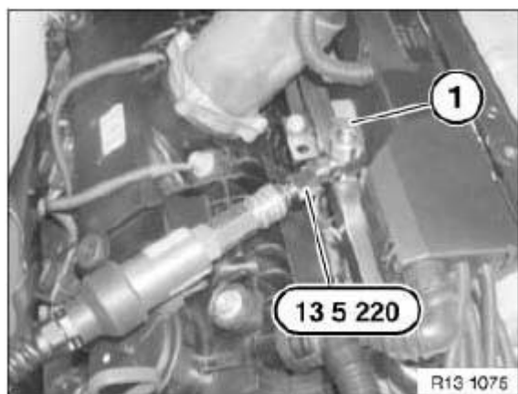
Fig. 1: Identifying Non-Return Valve On Special Tool (13 5 220)
