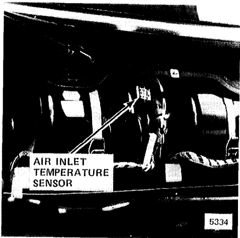
Figure 5 - Under Center Of Fresh Air Intake Cowl
