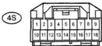
Fig. 103: Identifying 4Q, 4S Main Body ECU Connector Terminals Courtesy of TOYOTA MOTOR SALES, U.S.A., INC.
