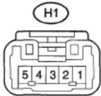
Fig. 8: Identifying Rear Power Window Regulator Switch Assembly LH Connector Terminals Courtesy of TOYOTA MOTOR SALES, U.S.A., INC.
