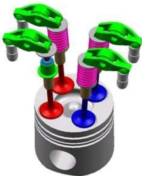
Fig. 19: Valve gear - M47/M57/M67
