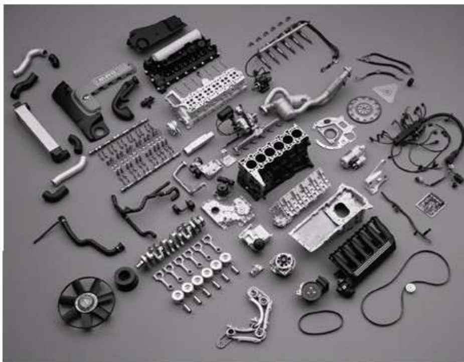
Fig. 10: Engine components and add-on parts - M57
