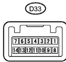
Fig. 5: D33 Engine Switch Connector Terminal Identification
