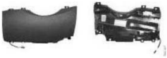
Fig. 21: Identifying E65 Driver Side Knee Airbag System Courtesy of BMW OF NORTH AMERICA, INC.
