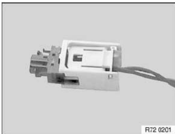
Fig. 26: Identifying Airbag Plug Connection Courtesy of BMW OF NORTH AMERICA, INC.
