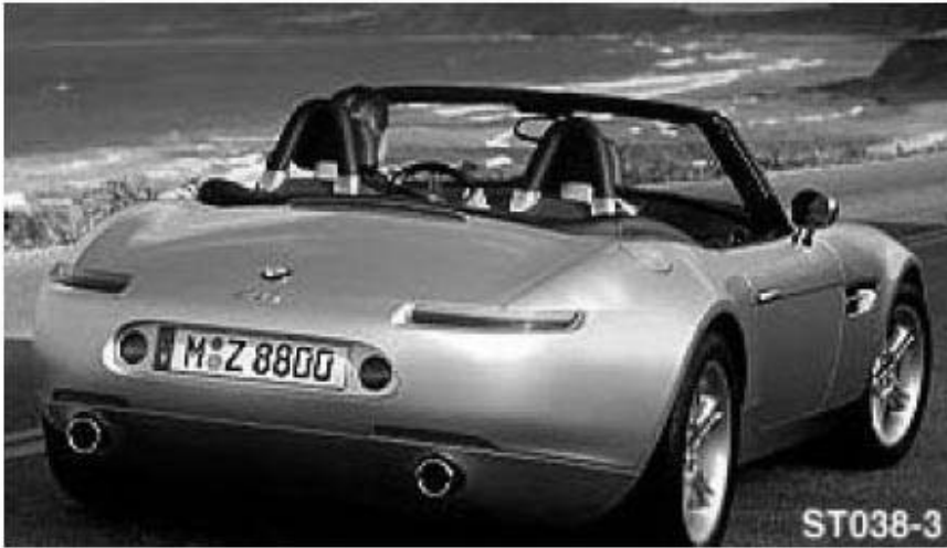
Fig. 25: Identifying Rollover Bars Courtesy of BMW OF NORTH AMERICA, INC.
