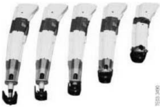
Fig. 8: Identifying Engine Support Arm System (1 Of 2) Courtesy of BMW OF NORTH AMERICA, INC.
