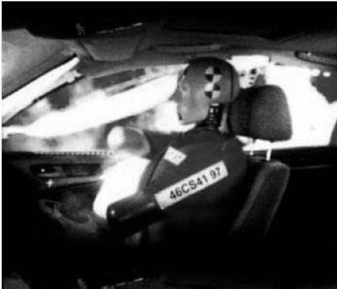
Fig. 17: Identifying Head Protection System Courtesy of BMW OF NORTH AMERICA, INC.
