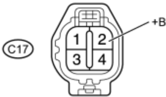
Front view of wire harness connector: (to HO2 Sensor for Bank 2)
