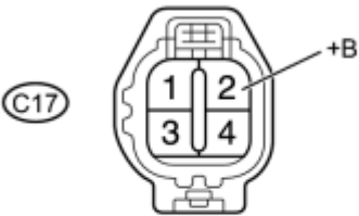
Front view of wire harness connector: (to HO2 Sensor for Bank 2)
