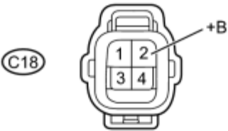
Front view of wire harness connector: (to Integration Relay)
