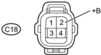
Front view of wire harness connector: (to HO2 Sensor for Bank 2)
