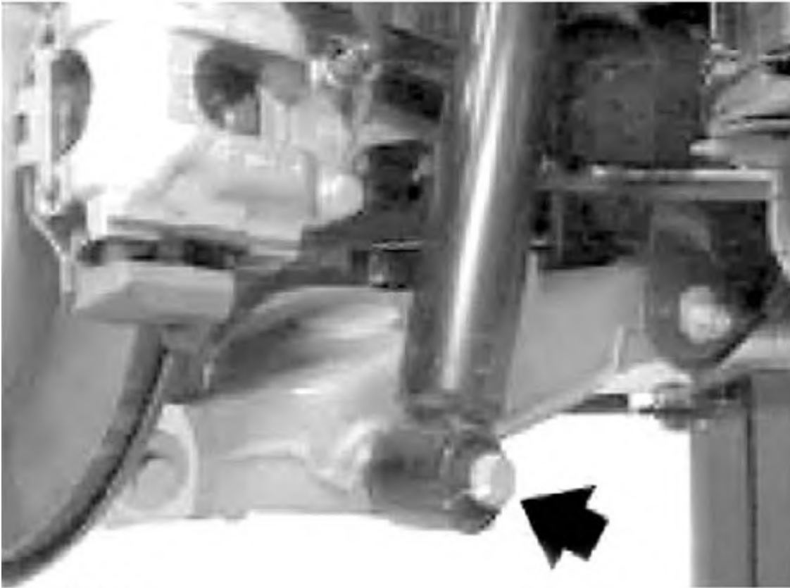
Fig. 27: Releasing Shock Absorber Courtesy of BMW OF NORTH AMERICA, INC.
