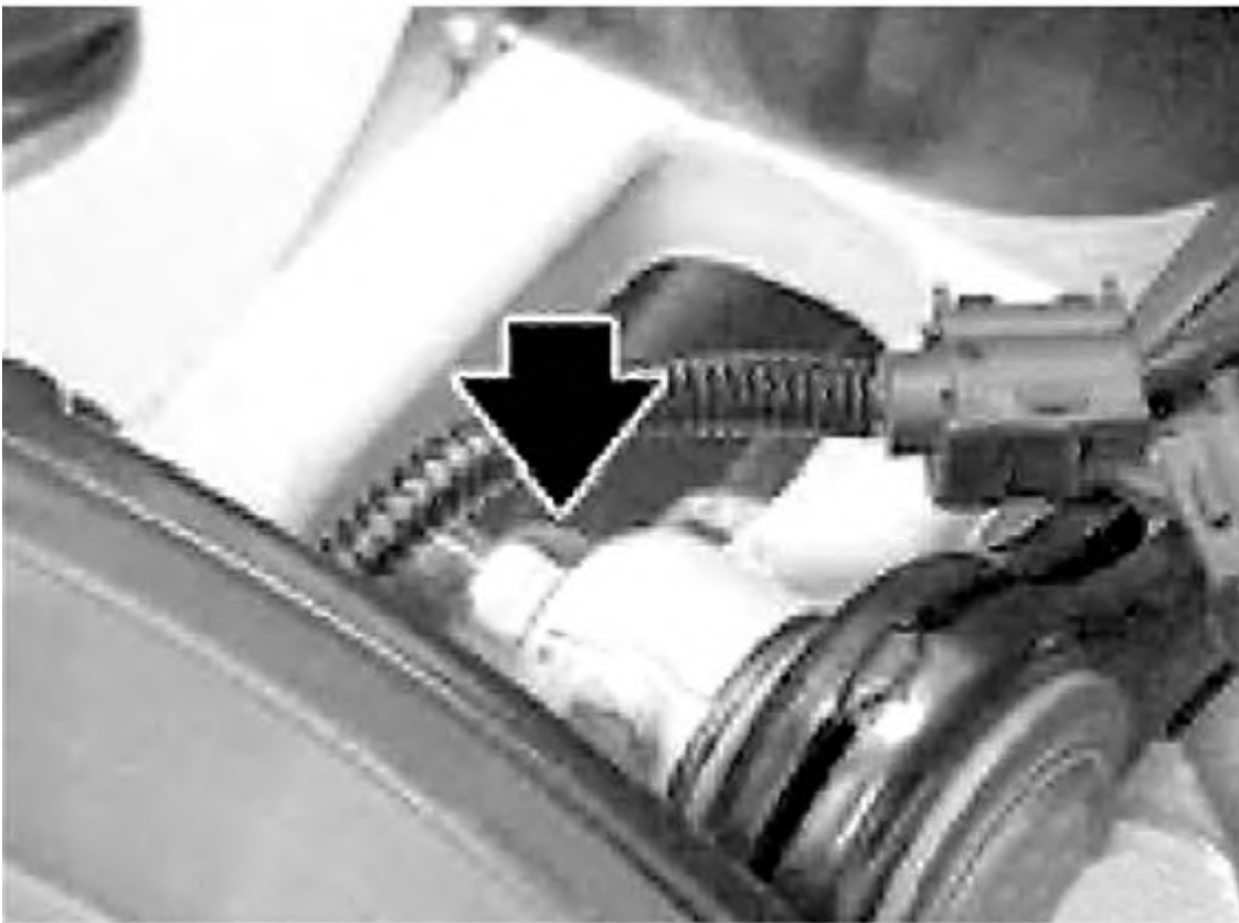
Fig. 37: Locating Nut For Upper Control Arm To Wheel Carrier Courtesy of BMW OF NORTH AMERICA, INC.
