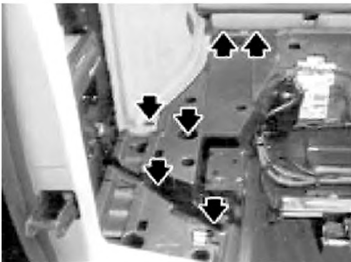
Fig. 24: Removing Luggage Compartment Trim On Left Courtesy of BMW OF NORTH AMERICA, INC.
