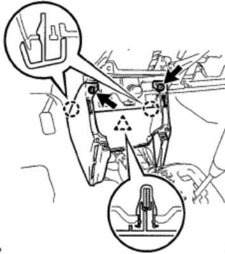
Fig. 46: Identifying Front Console Box Clip And Claws Courtesy of TOYOTA MOTOR SALES, U.S.A., INC.
