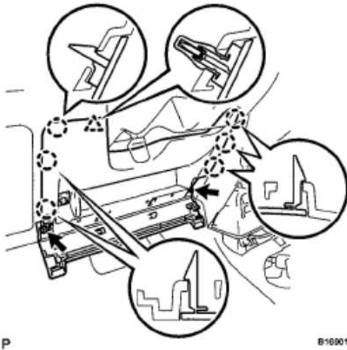
Fig. 79: Identifying Instrument Panel Under Tray Clip And Claws Courtesy of TOYOTA MOTOR SALES, U.S.A., INC.
