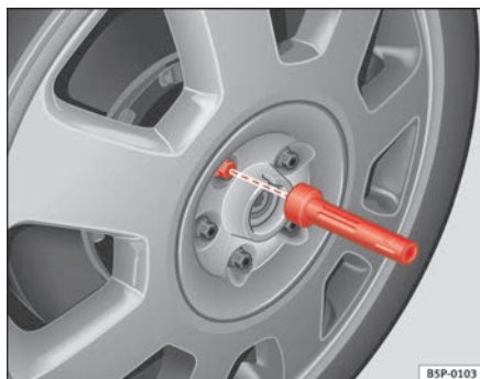
Fig. 136 Changing the wheel: hexagonal socket in screwdriver handle to turn the wheel bolts after they have been loosened
