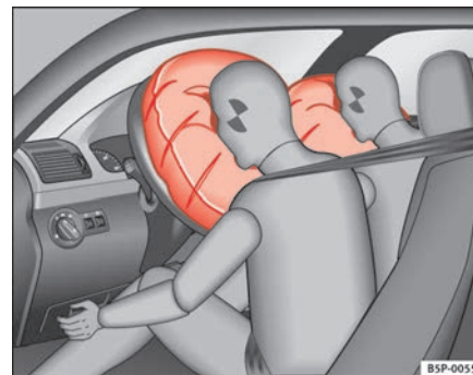
Fig. 19 Inflated front airbags
