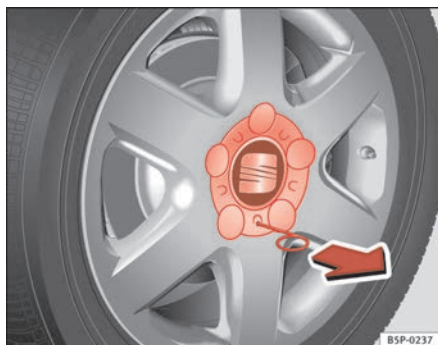
Fig. 131 Changing the wheel: Removing a hub cap
