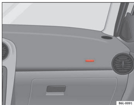
Fig. 18 Front passenger airbag located in dash panel
