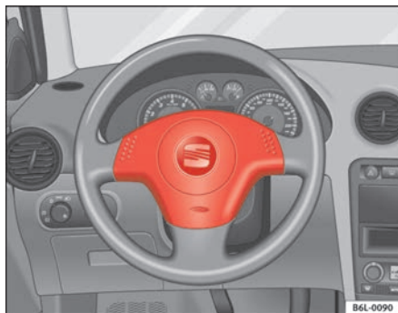
Fig. 17 Driver airbag located in steering wheel
