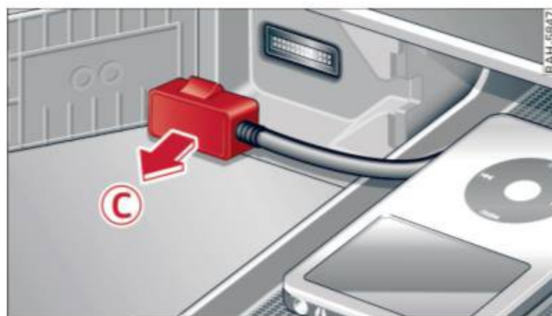
Fig. 10 Adapter cable: Removing the released jack from the Audi music interface
