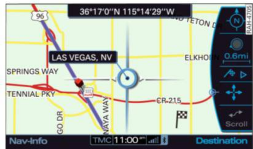
Fig. 59 Changing the destination with the crosshairs
