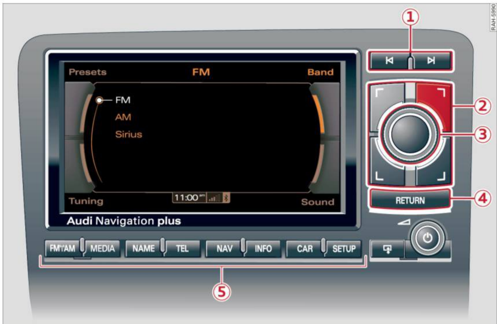
Fig. 14 Buttons on the control panel
