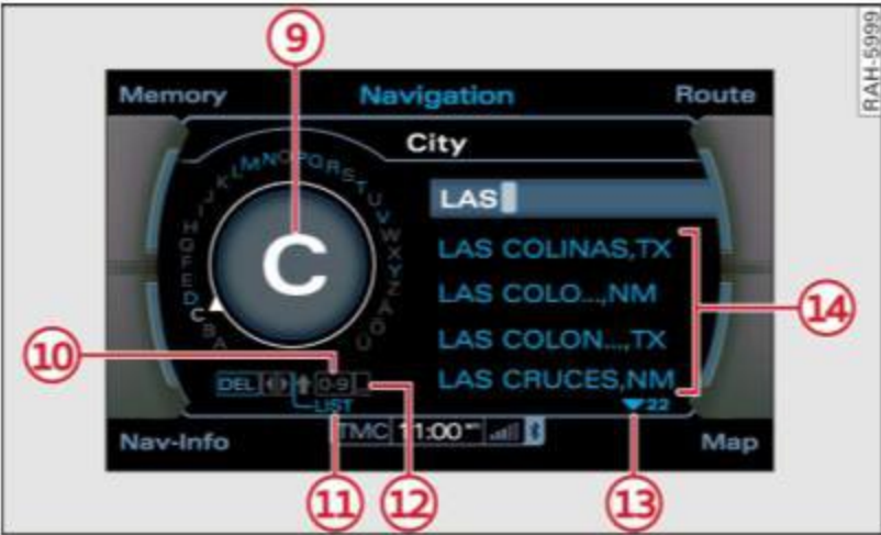
Fig. 18 Letter speller: Entering a navigation destination
