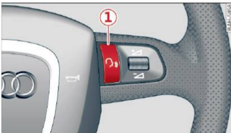
Fig. 73 Multifunction steering wheel: Talk button
