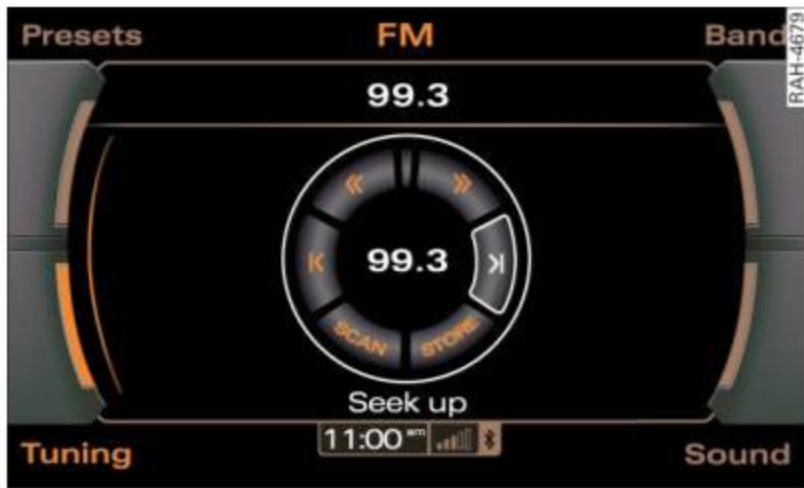
Fig. 34 Automatic station search forward (FM band)
