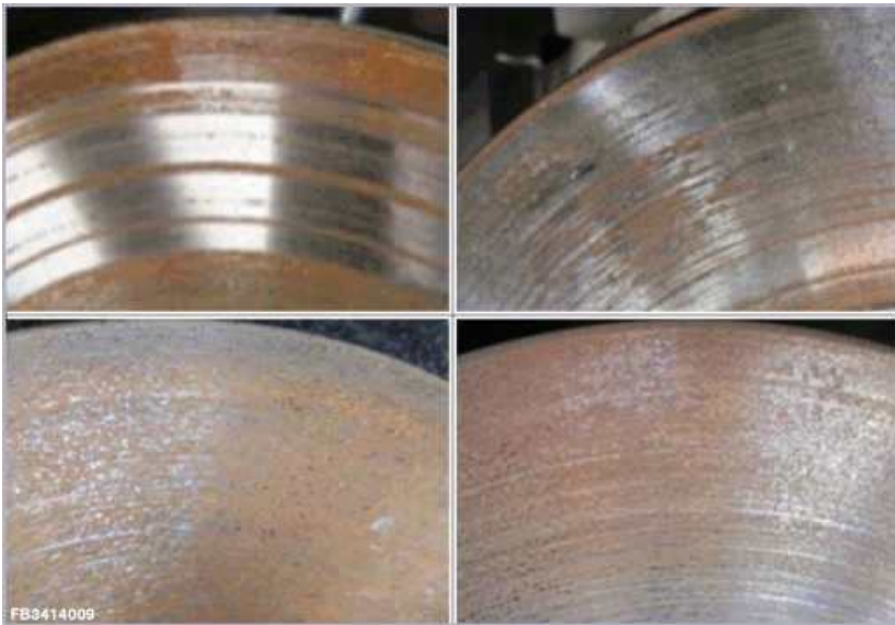
Figure shows faulty brake discs due to corrosion.
