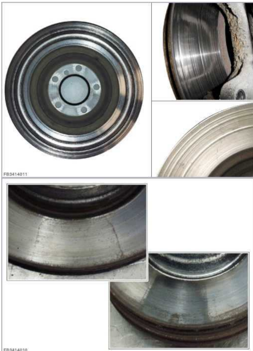
Figure shows faulty brake discs due to corrosion.
