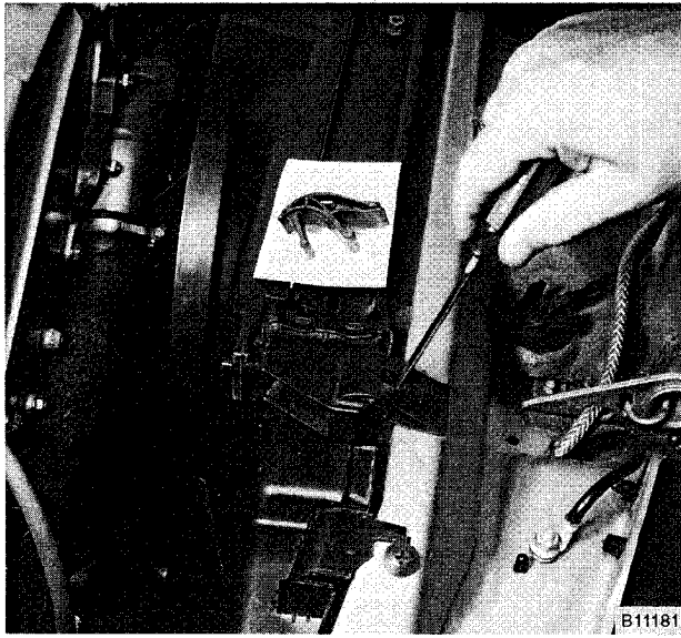
Fig. 22. Radiator retaining clip being removed. Push down and pull screwdriver forward to release clip.
