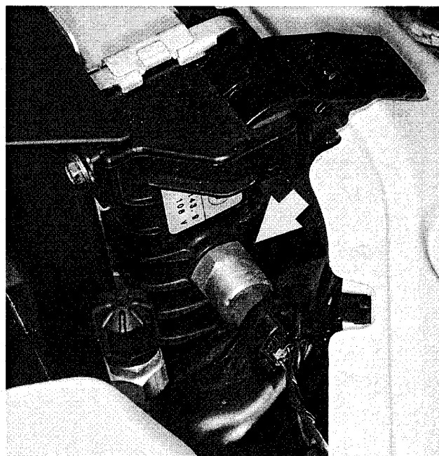
Fig. 3. Radiator cooling fan temperature switch (arrow).
