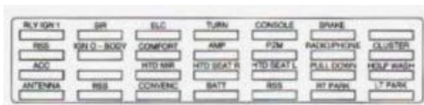
Cadillac Eldorado – fuse box diagram – rear
